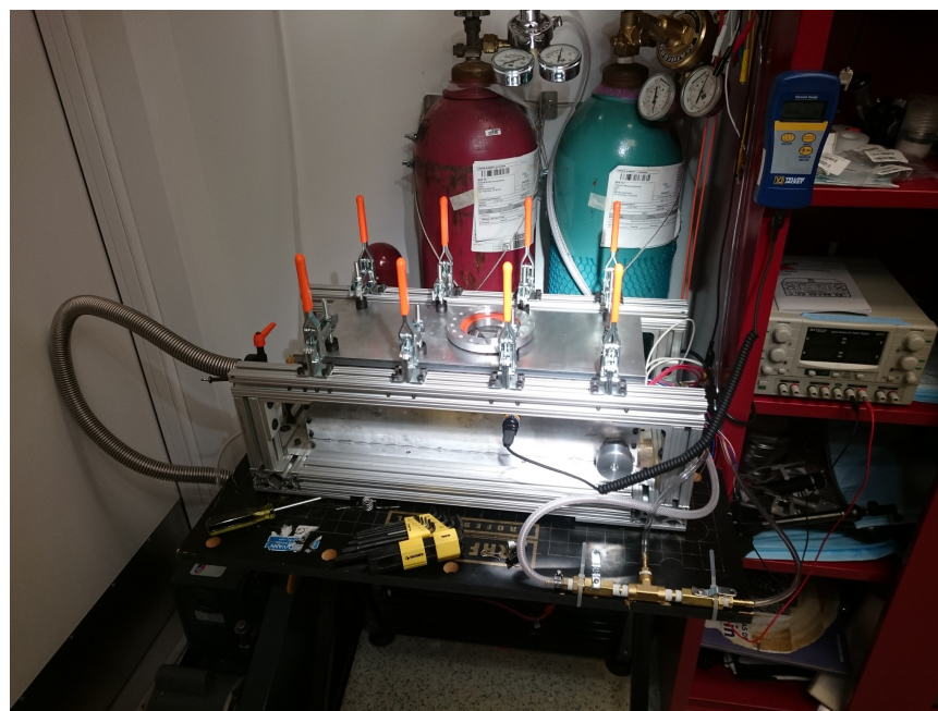
Figure 14: Photograph of the assembled, working needle brazing machine.
